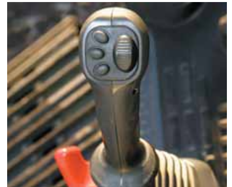
Joysticks with proportional control button for attachments
